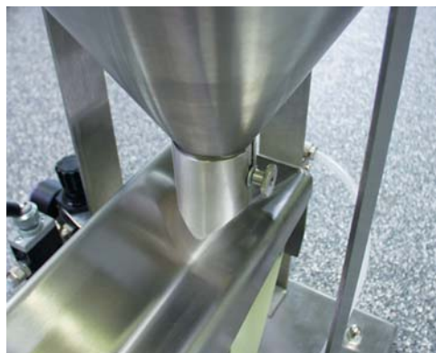
Dosing port at the silo outlet
