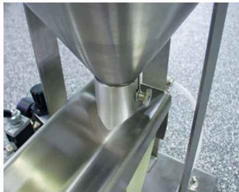
Dosing port at the silo outlet
