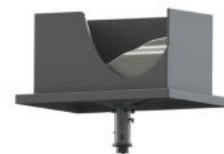
NHK 25 on vibrating table
