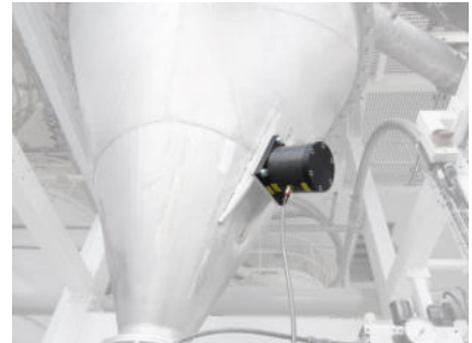
NTS 54/02 for improving material flow
