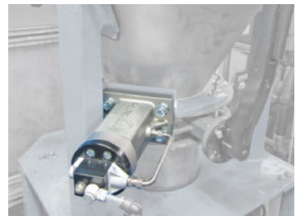
PKL 740 for loosening bridge formations
