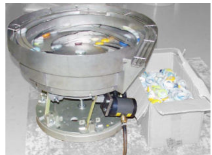
NTS 100/01 for spiral conveying of bulk materials
