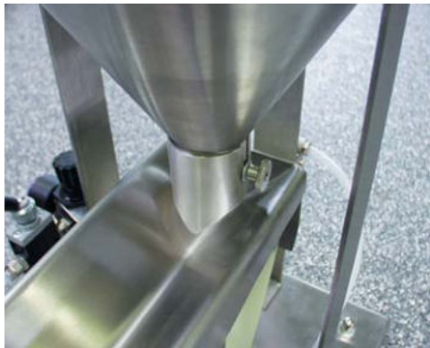
Dosing port at the silo outlet
